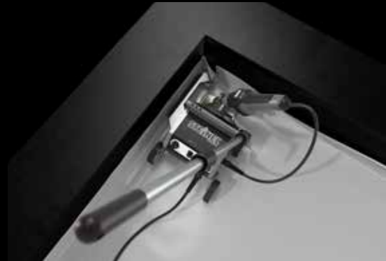
Welding as close as 8 cm to the edge on straight sides.
