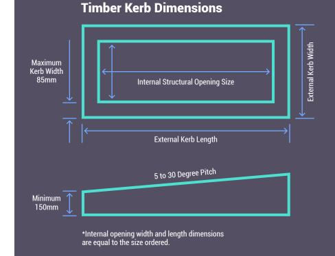
Example of a 5-degree minimum pitch: This equates to a grade of 1:11.5. E.g. a roof light with 1000mm width will require a fall of 87mm.
